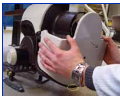
Fig. 3-2 Service kap demonteren
