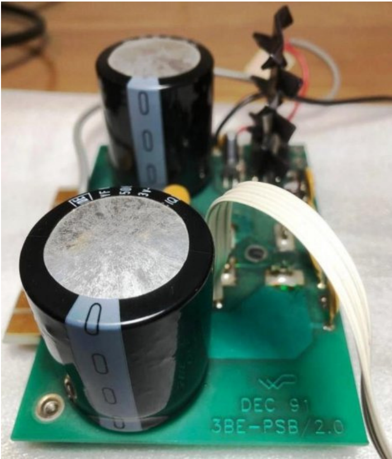
Figure 4. Original dual capacitors fitted to each channel, RDE 7,500 \mu\text{F} , 63 V (note board markings Dec 91, 3BE-PSB/2.0).
