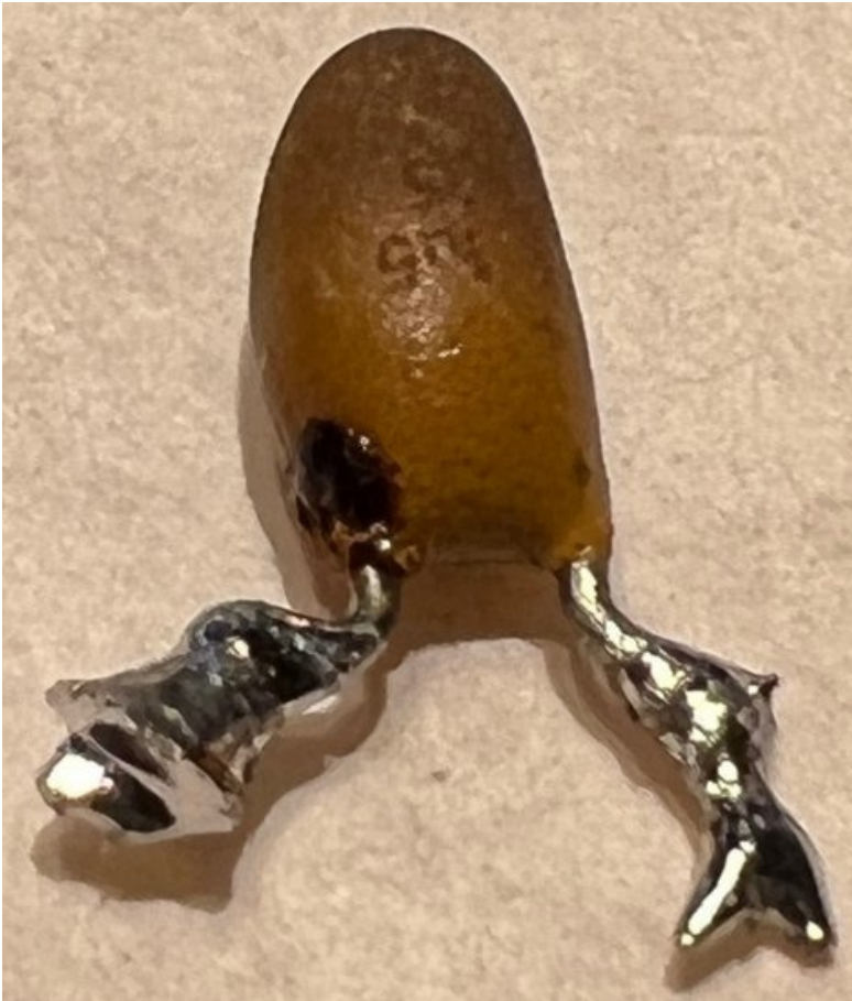
Figure 9. Two tantalum capacitors on either side of the black axial capacitor, closeup of a removed tantalum burnt/leaking.
