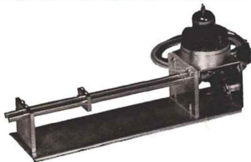
Fig. 8. Experimental test arrangement for Z-2061 magnetron
