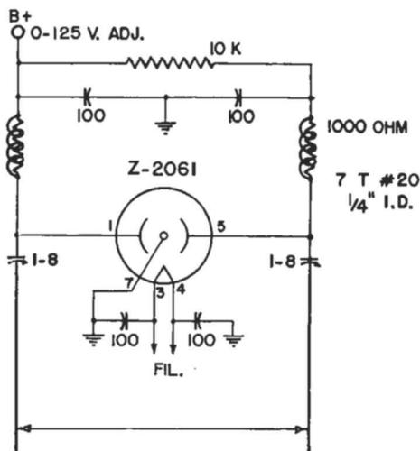
Fig. 10. Circuit diagram of Z-2061 test set
