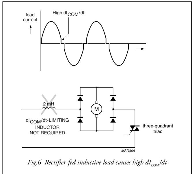
Fig.6 Rectifier-fed inductive load causes high  $dI_{COM}/dt$
