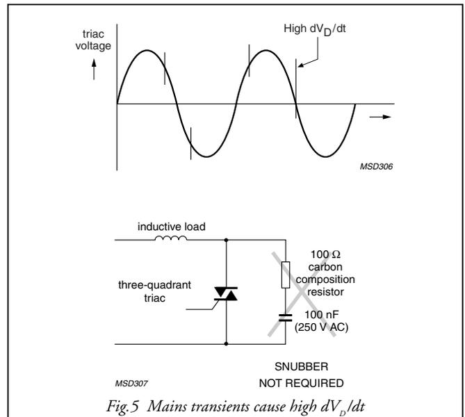
The removal of the triac's critical overlapping feature mentioned previously has given Philips' Hi-Com triacs a minimum  $dV_D/dt$  capability of 1000 V/ $\mu$ s and a typical capability of 4000 V/ $\mu$ s.
