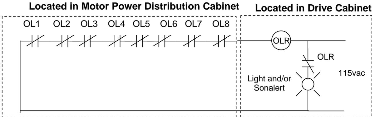
If you wish to trip the drive if one of the motor overloads trip, you could do the following: the Drive will annunciate with **Et** External Trip
