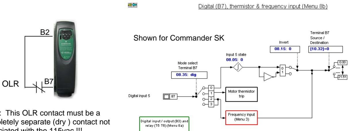
**Note:** This OLR contact must be a completely separate (dry ) contact not associated with the 115vac !!!
