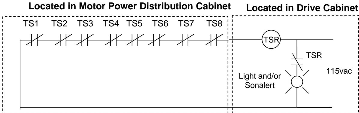
If you wish to trip the drive if one of the motor overloads trip, you could do the following: the Drive will annunciate with **EE** External Trip
