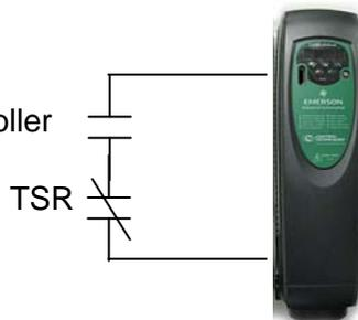
Obviously, should a Thermostat trip, the drive would drop out of run **BUT** as soon as the motor cooled down the drive would re-start at that time which may not be a safe condition. In these cases, it would be best that the controller be cognizant of the Thermostat state(s) and handle the RUN command appropriately.
