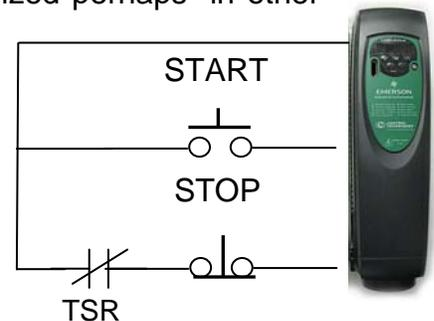
You would **not** want to place this contact in series with a Run contact from a Control System however.
