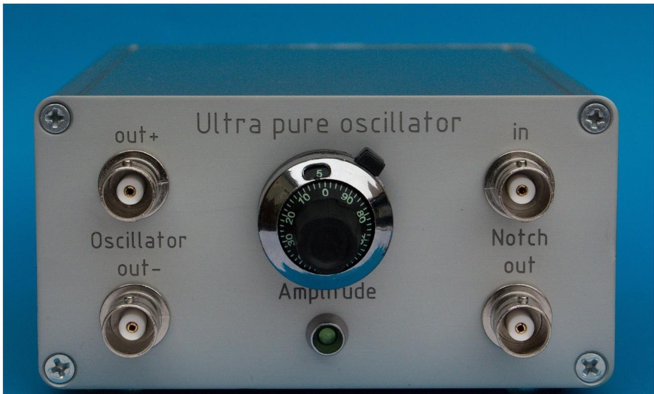
Fig. 9. A complete oscillator
