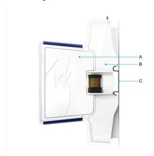
Module (A) and base (B) form a unique combination. As a result of this, a module cannot be incorrectly positioned in a base.
