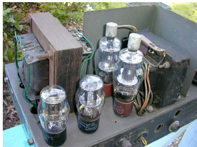
OT sandwiched between output valves and barriers.
