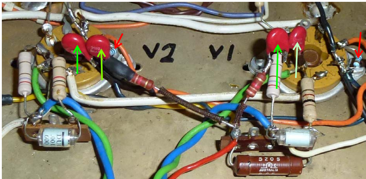
Figure 9. Ultra-linear PP stage (RTV&H 1960 100W PA amp). Original RC network from plate to screen. 1 \Omega cathode sense resistors added. Series MOV-R circuit added to each primary half. No screen stoppers added.
