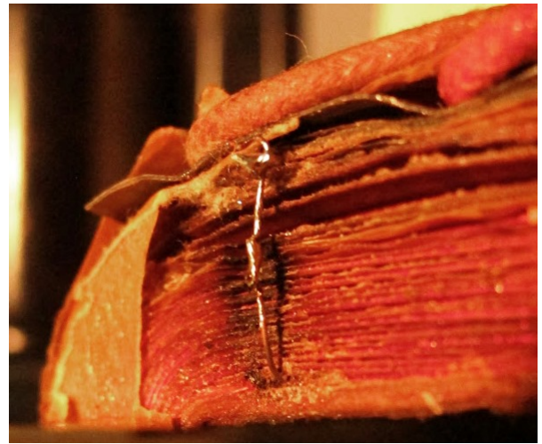
Figure 11. Repairable fault in output transformer.
