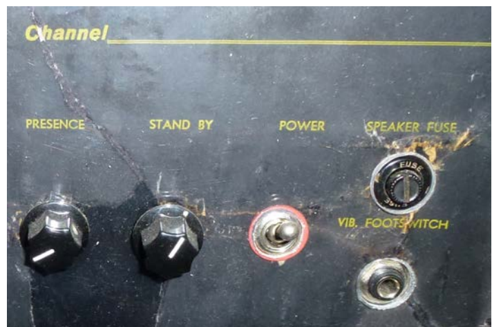
Speaker fusing is not common – with good reason!
