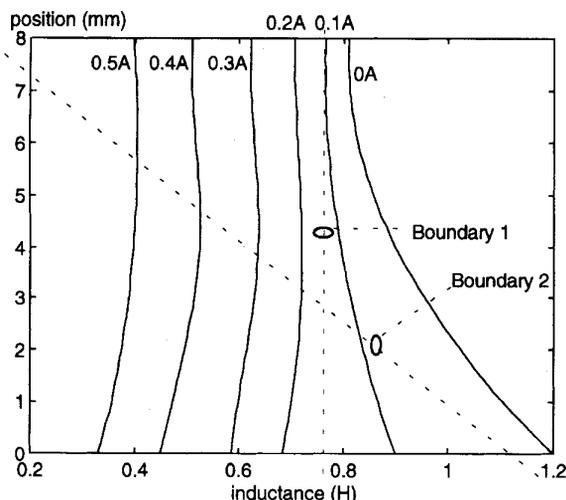
Fig. 5. Variation of incremental inductance with position at different levels.
