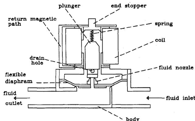
Fig. 1. Construction of a two-stage solenoid valve.
