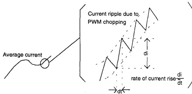
Fig. 3. Measuring  $di/dt$  from a PWM current waveform.
