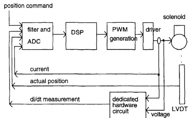
Fig. 8. Setup of the position estimation experiment.
